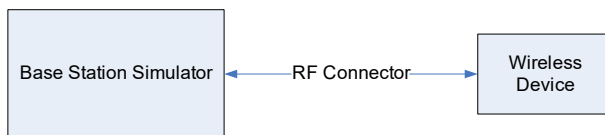
Figure 10-1 Power Measurement Setup – NR FDD
