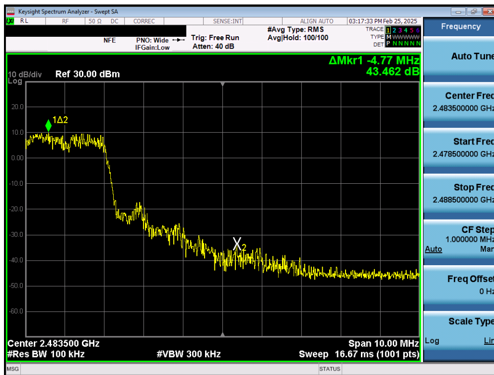
Plot 7-124. Band Edge Plot (Bluetooth with Hopping Enabled, 3 Mbps) – Dual Ant 2
