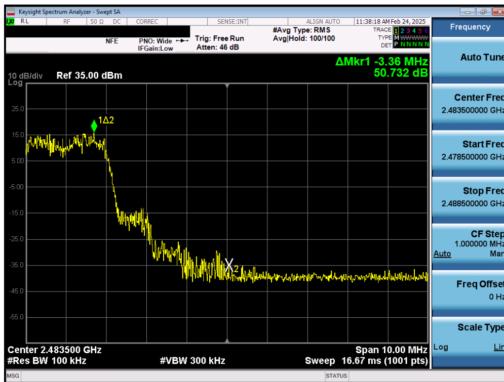
Plot 7-112. Band Edge Plot (Bluetooth with Hopping Enabled, 3 Mbps) – Ant 1
