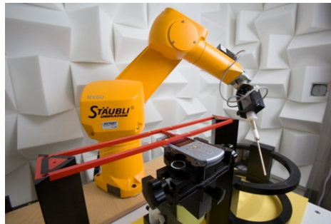
Figure 4-3 SPEAG Robotic System
