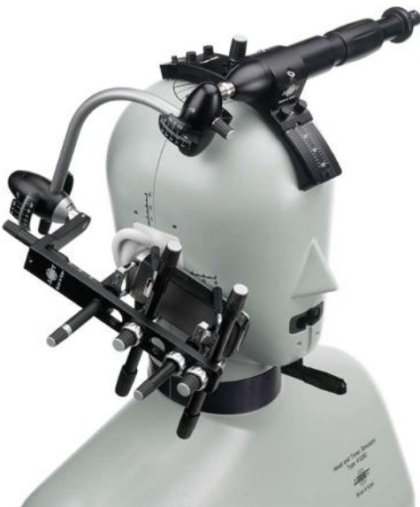
Figure 4-3 Heat and Torso Simulator (with Handset Positioner)
