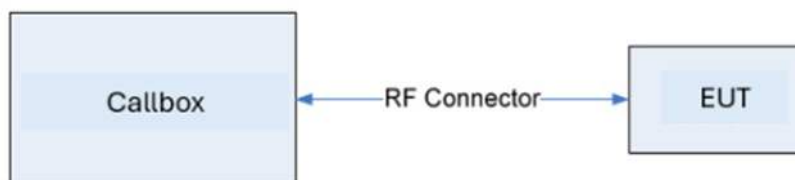
Figure 6-1. Test Instrument & Measurement Setup
