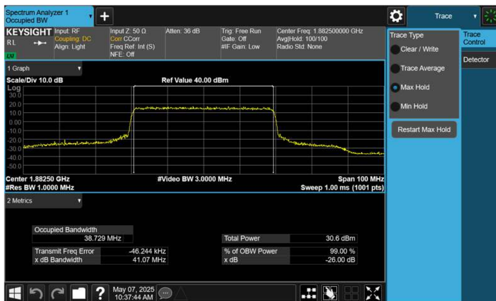
Plot 6-5. Occupied Bandwidth Plot (NR Band n25/2 - 40.0MHz CP-OFDM 16QAM - Full RB - ANT2)
