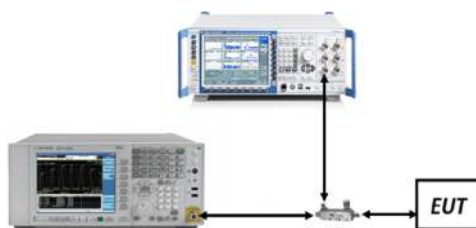
Figure 6-2. Test Instrument & Measurement Setup
