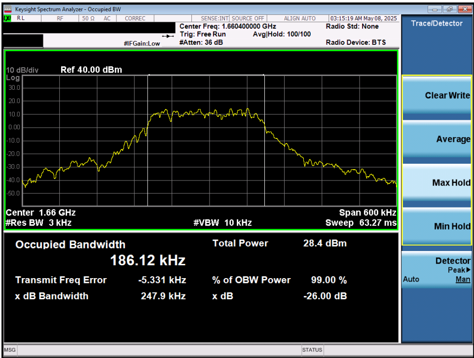
Plot 6-3. Bandwidth Plot (Band n255, High Channel)
