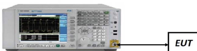
Figure 6-3. Test Instrument & Measurement Setup
