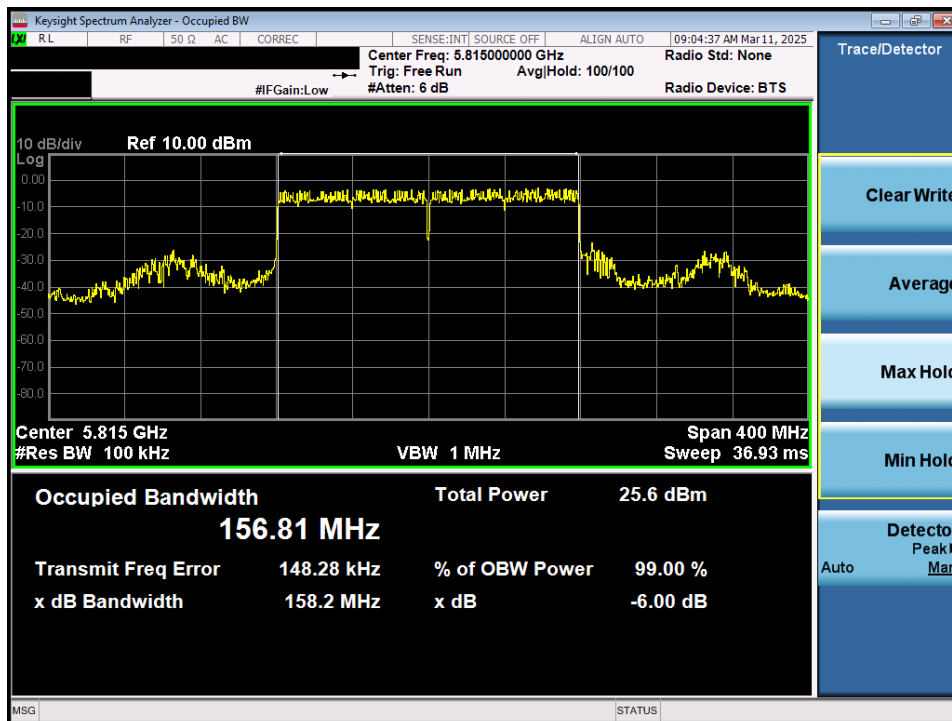
Plot 7-41. 6dB Bandwidth Plot MIMO ANT1 (160MHz 802.11ax/be (Full Tones) (UNII Band 3/4) – Ch. 163)
