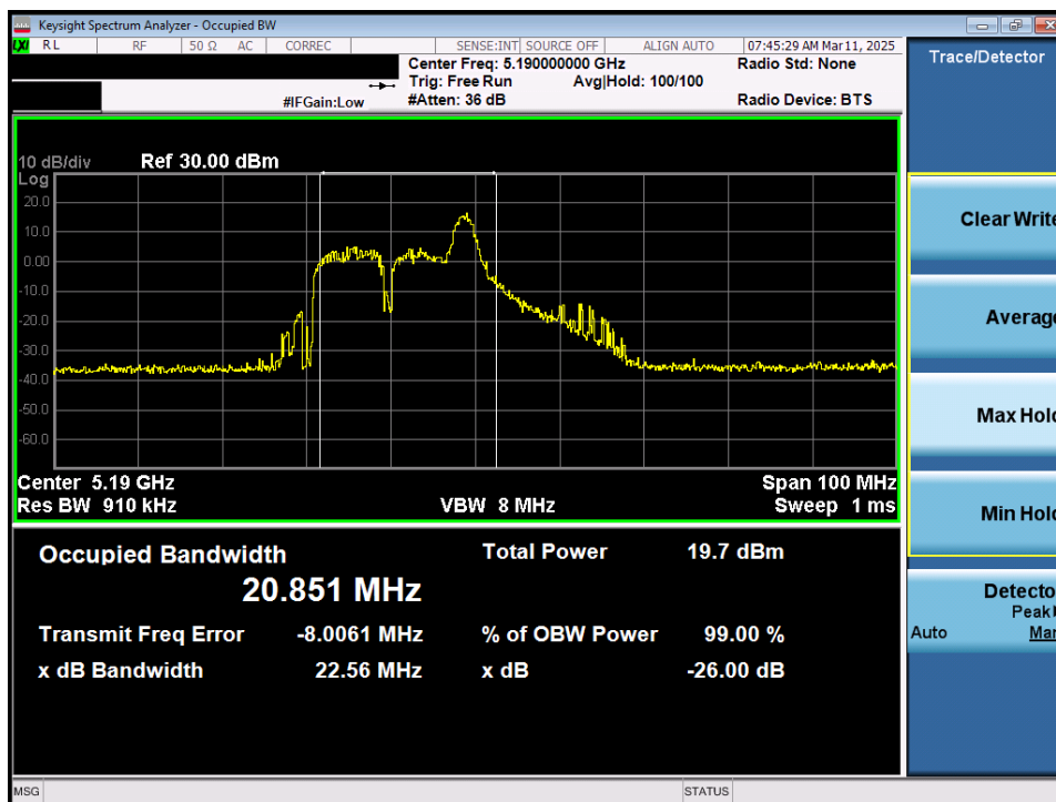
Plot 7-2. 26dB Bandwidth Plot MIMO ANT1 (40MHz 802.11ax/be (26 Tones) (UNII Band 1) – Ch. 38)
