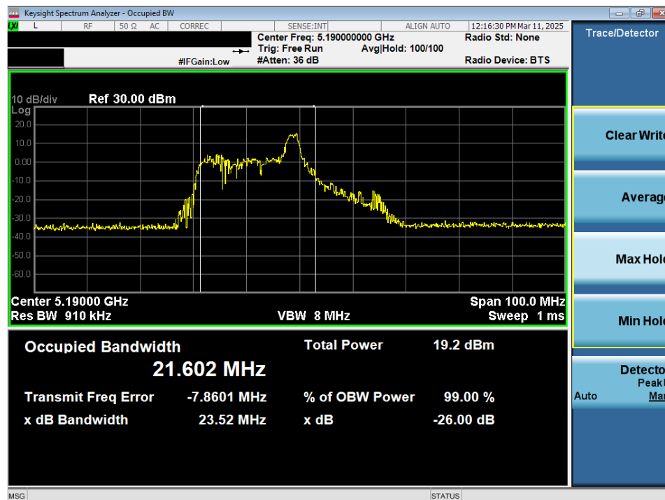
Plot 7-13. 26dB Bandwidth Plot MIMO ANT2 (40MHz 802.11ax/be (26 Tones) (UNII Band 1) – Ch. 38)
