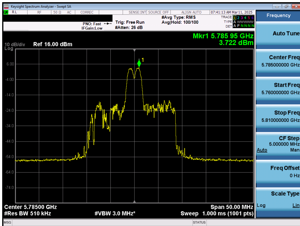
Plot 7-72. Power Spectral Density Plot MIMO ANT1 (20MHz 802.11ax/be (26 Tones) (UNII Band 3) – Ch. 157)
