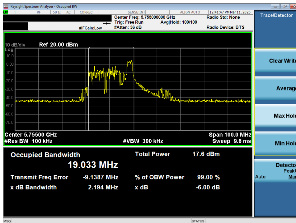
Plot 7-43. 6dB Bandwidth Plot MIMO ANT2 (40MHz 802.11ax/be (26 Tones) (UNII Band 3) – Ch. 151)
