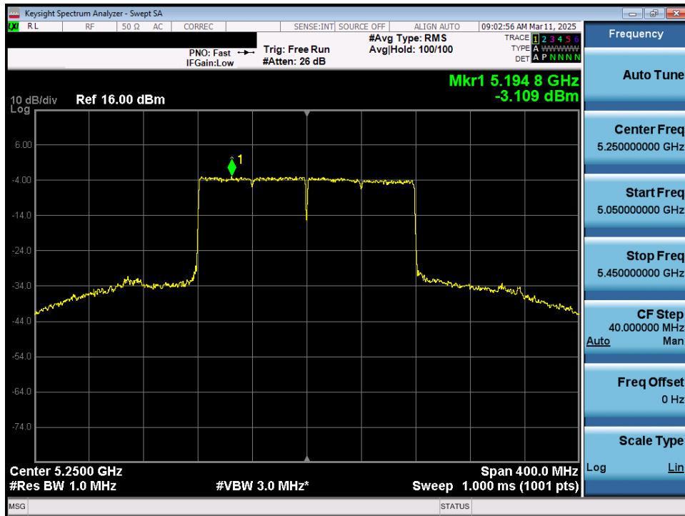
Plot 7-71. Power Spectral Density Plot MIMO ANT1 (160MHz 802.11ax/be (Full Tones) (UNII Band 1/2A) – Ch. 50)
