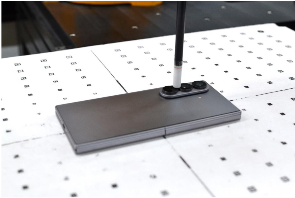
PD Test Setup Photo 43 – PD, Closed Back Side at 2mm
