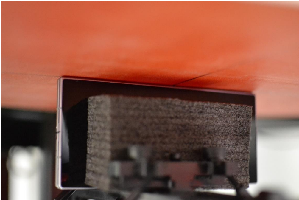
SAR Test Setup Photo 35 – NFC Phablet, Folder Closed, Left Edge at 0mm
