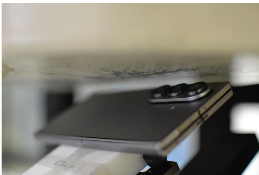
SAR Test Setup Photo 10 – Body-worn/Hotspot, Folder Closed, Back Side at 5mm (for Antenna H)
