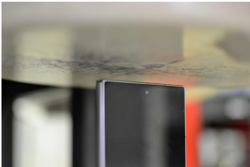
SAR Test Setup Photo 17 – Hotspot, Folder Closed, Top Edge at 10mm
