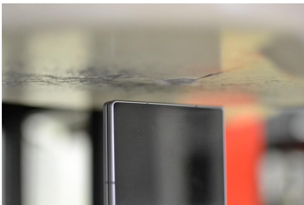
SAR Test Setup Photo 14 – Hotspot, Folder Closed, Bottom Edge at 10mm
