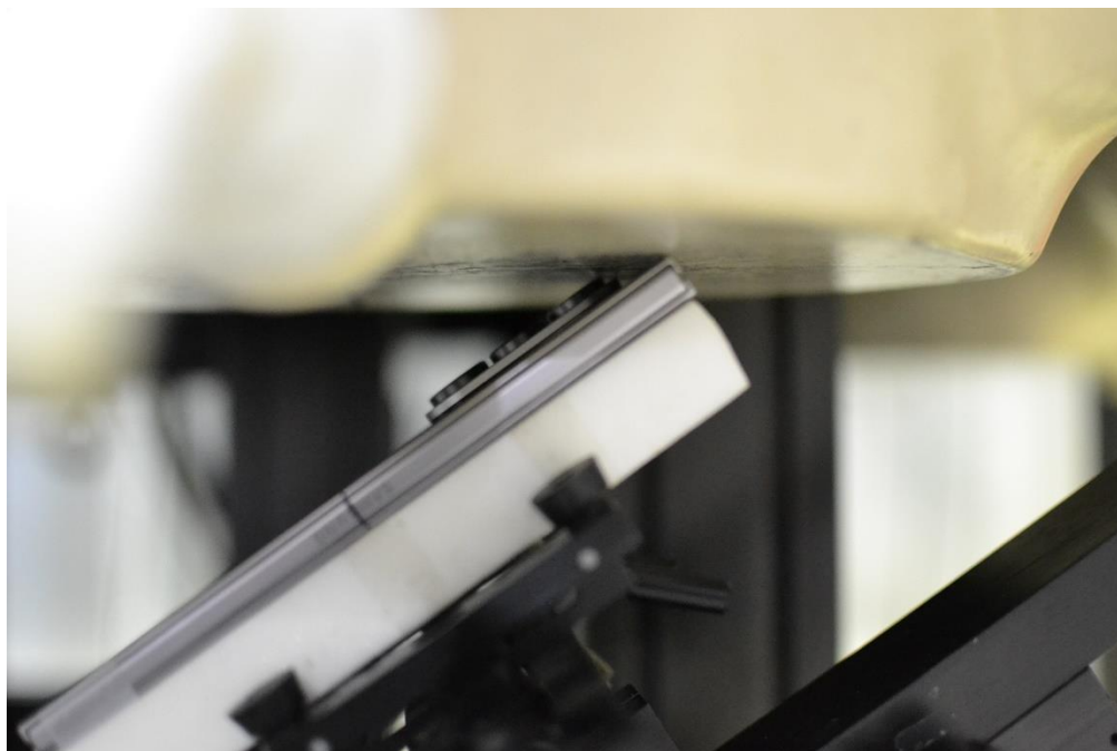
SAR Test Setup Photo 9 – Phablet, Folder Closed, Back Side at 0mm (for AG1)
