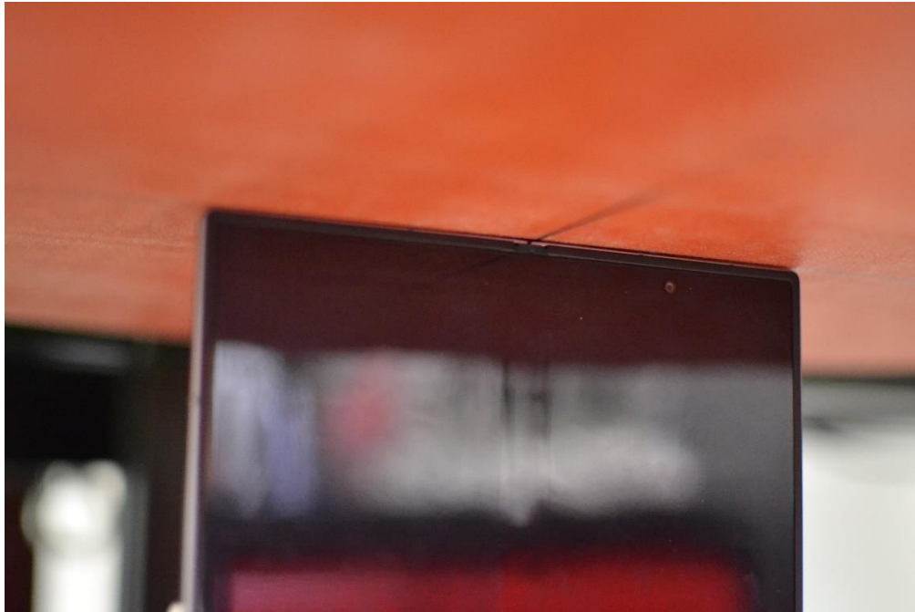
SAR Test Setup Photo 37 – NFC Tablet, Folder Open, Top Edge at 0mm
