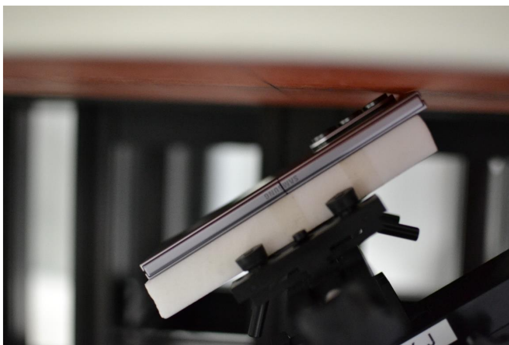
SAR Test Setup Photo 32 – NFC Phablet, Folder Closed, Back Side at 0mm
