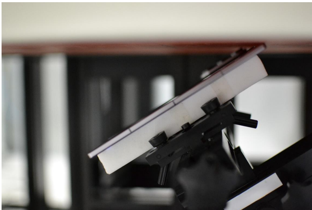
SAR Test Setup Photo 36 – NFC Tablet, Folder Open, Back Side at 0mm
