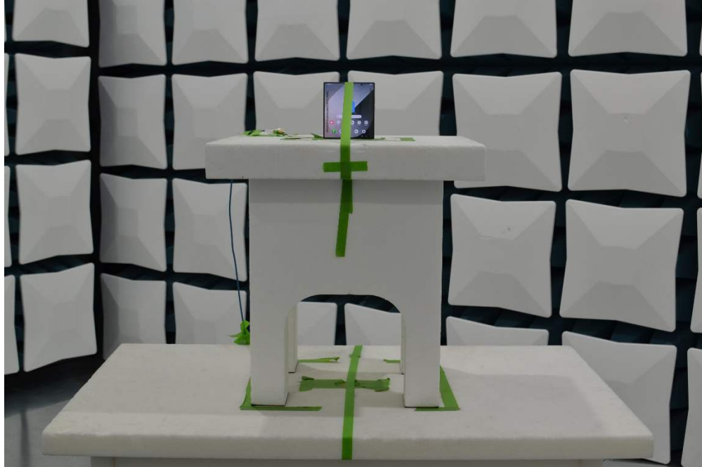
Figure 7. Test Setup – Z Position – 1GHz-40GHz – Open
