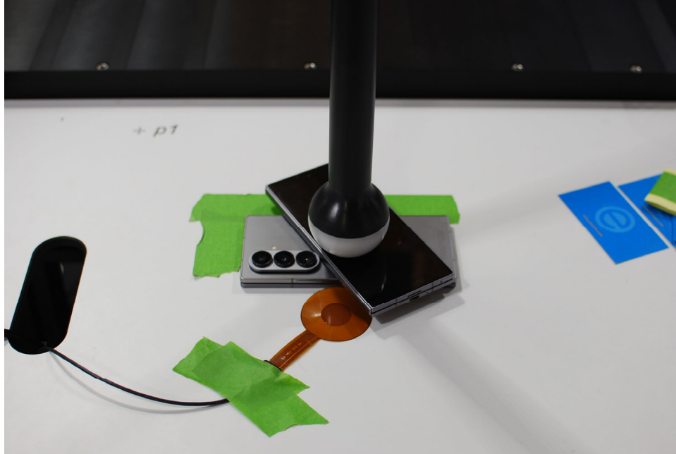
Test Setup Photo 9 Device to Device - Offset, Folder Closed, Back Side, 0mm
