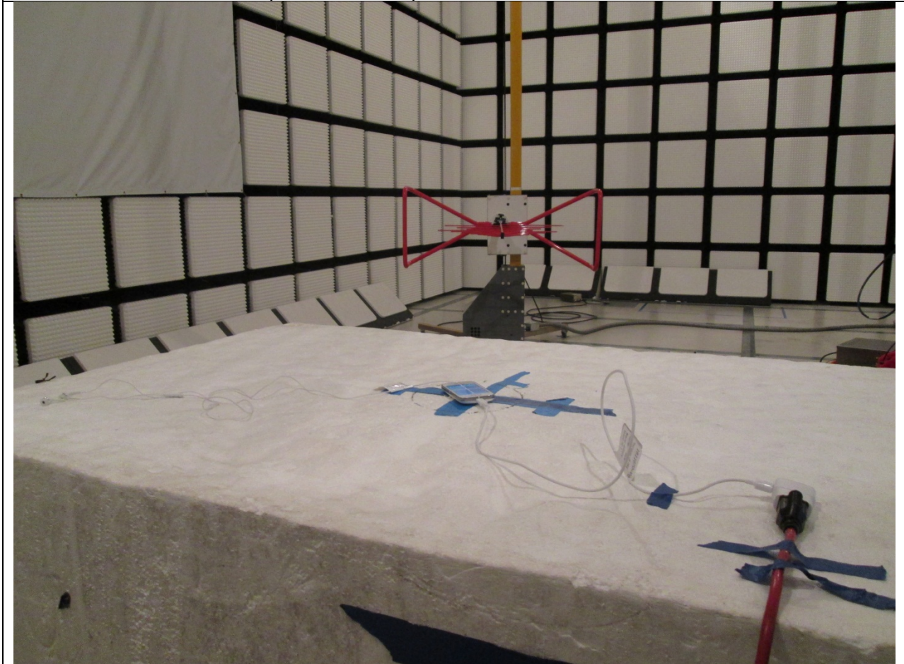
RADIATED BACK PHOTO (BELOW 1 GHz)
