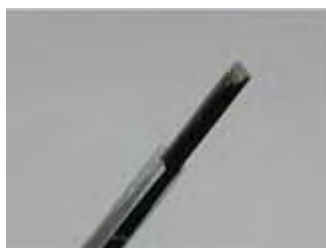
Figure 6. EX3DV4 E-field Probe
