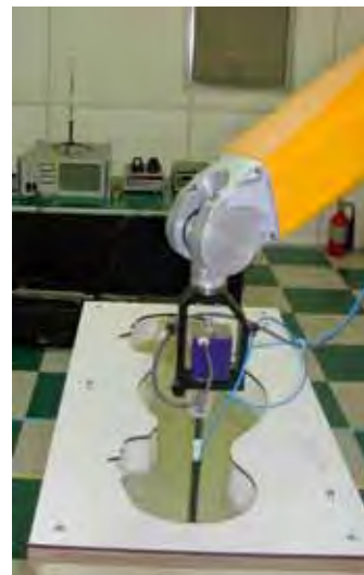
Figure 3. Photograph of the probe and the Phantom
