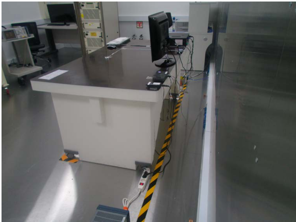
[ Conducted Disturbance – Rear ]
