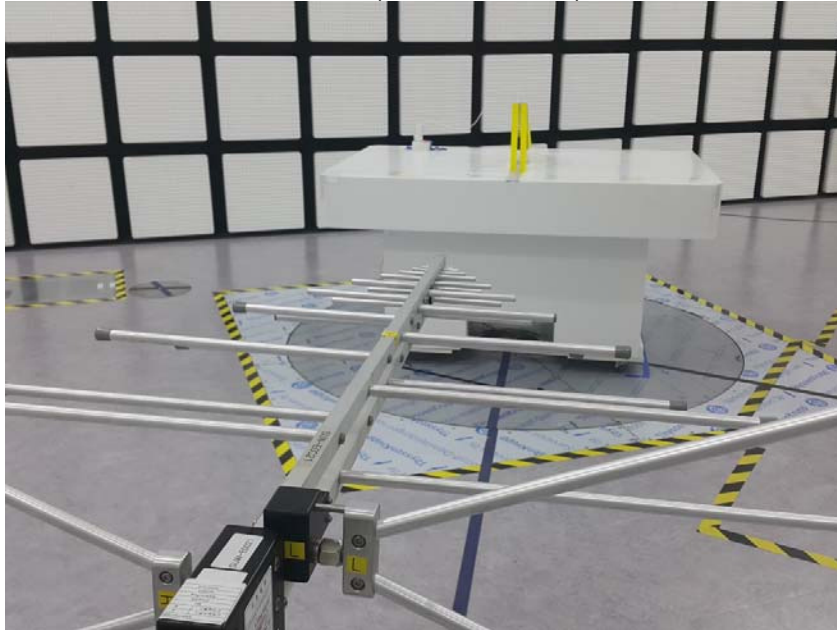
RADIATED FRONT PHOTO (BELOW 1 GHz)
