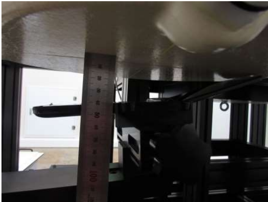
[Distance of 4.0 cm from the EUT]
