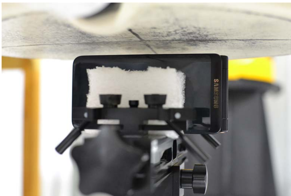
SAR Test Setup Photo 10 – Left at 1.0 cm
