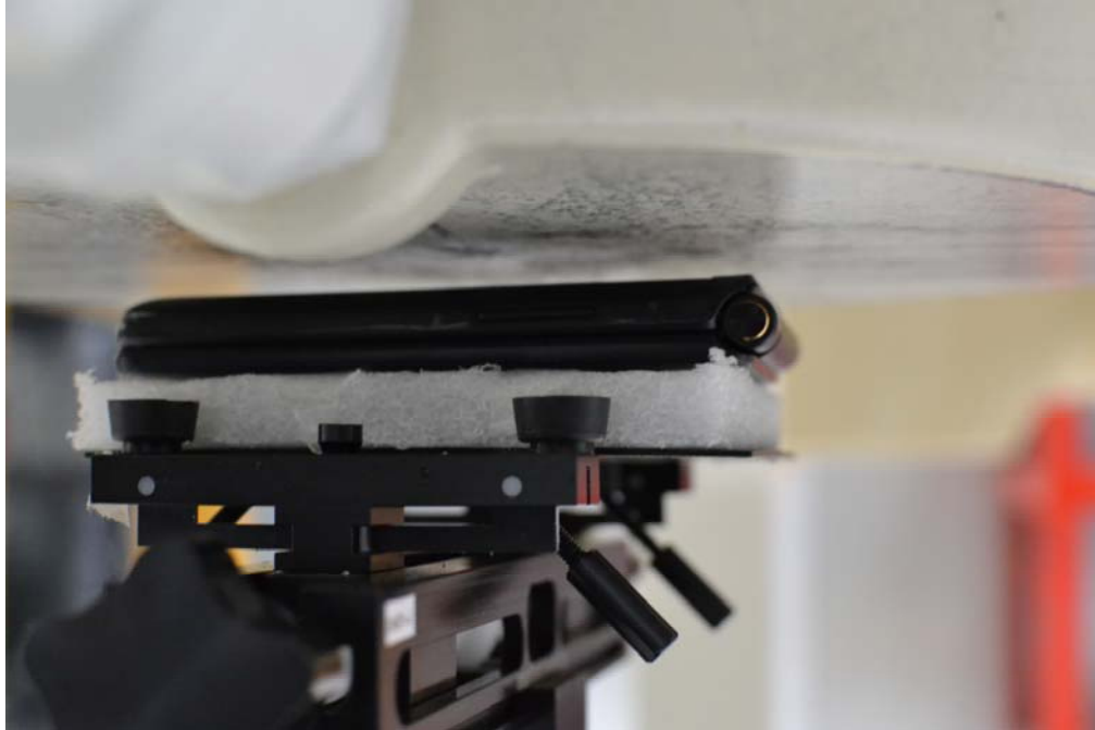
SAR Test Setup Photo 5 – Back at 1.0 cm
