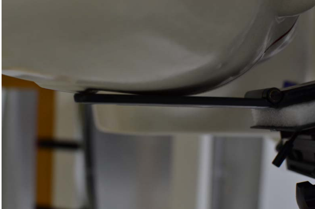
SAR Test Setup Photo 1 – Right Cheek
