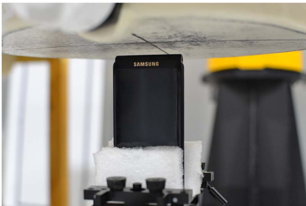
SAR Test Setup Photo 7 – Top at 1.0 cm
