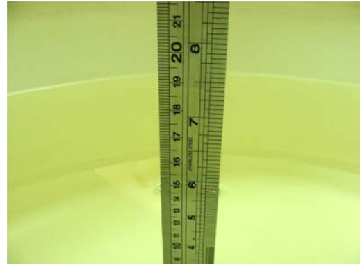
Photo of Liquid Height for Body SAR
