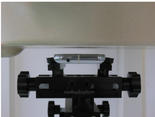
Front, Test Separation 1 cm
