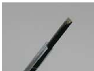
Figure 6. EX3DV4 E-field Probe
