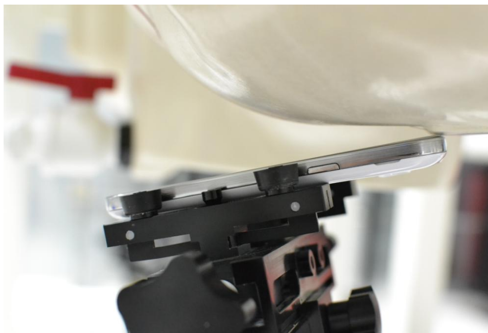
SAR Test Setup Photo 4: Left Tilt
