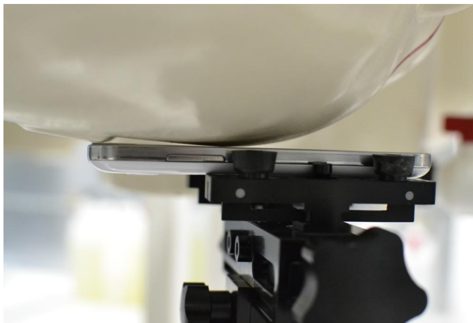
SAR Test Setup Photo 1: Right Cheek
