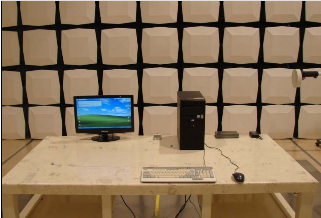
[ Radiated Disturbance for Below 1 GHz – Front ]
