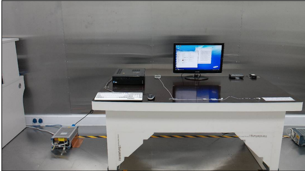
[ Conducted Disturbance – Front ]
