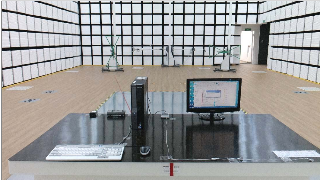
[ Radiated Disturbance for Below 1 GHz – Front ]
