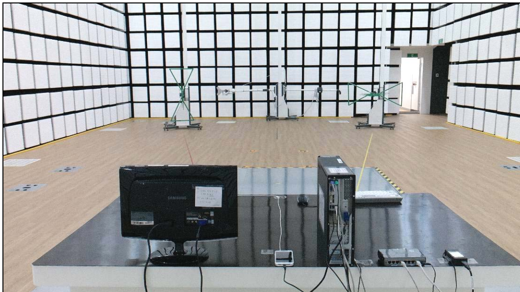
[ Radiated Disturbance for Below 1 GHz – Rear ]
