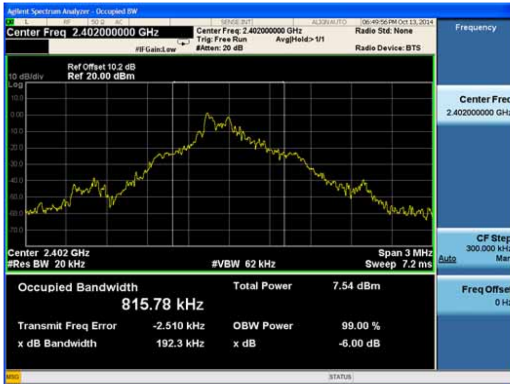
Occupied Bandwidth plot (Low-CH 0)
