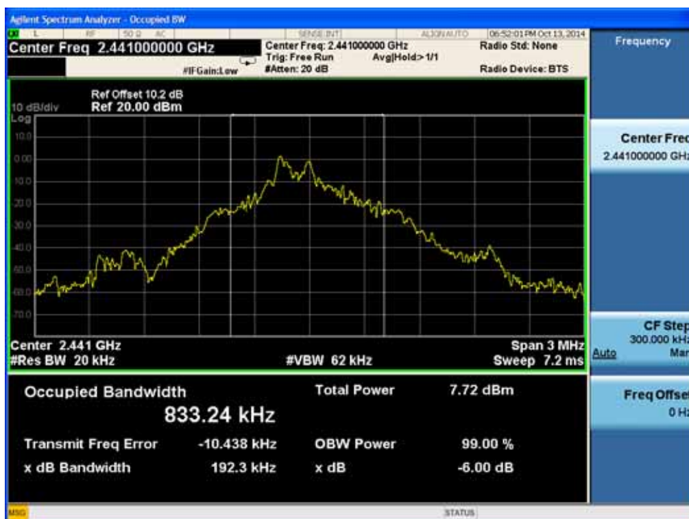
Occupied Bandwidth plot (Mid-CH 39)
