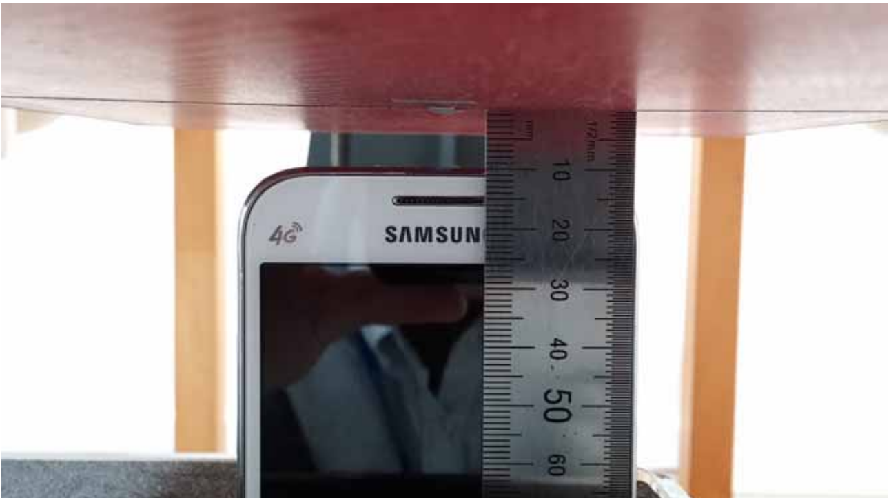
[Distance of 1.0 cm from the EUT]
