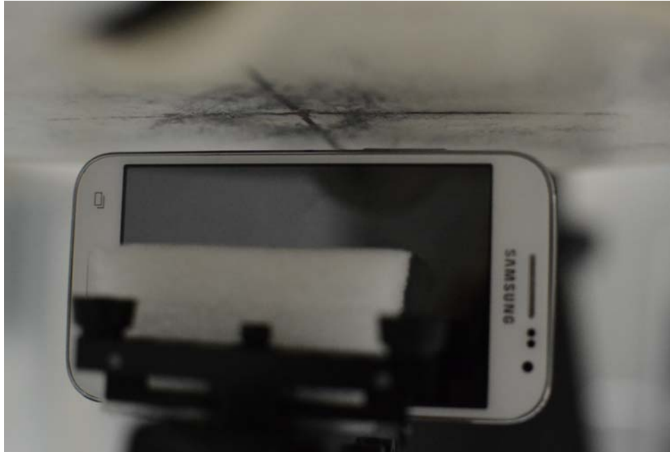
SAR Test Setup Photo 10: Left at 1.0 cm
