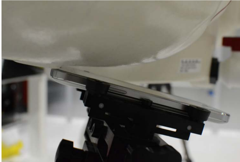
SAR Test Setup Photo 2: Right Tilt
