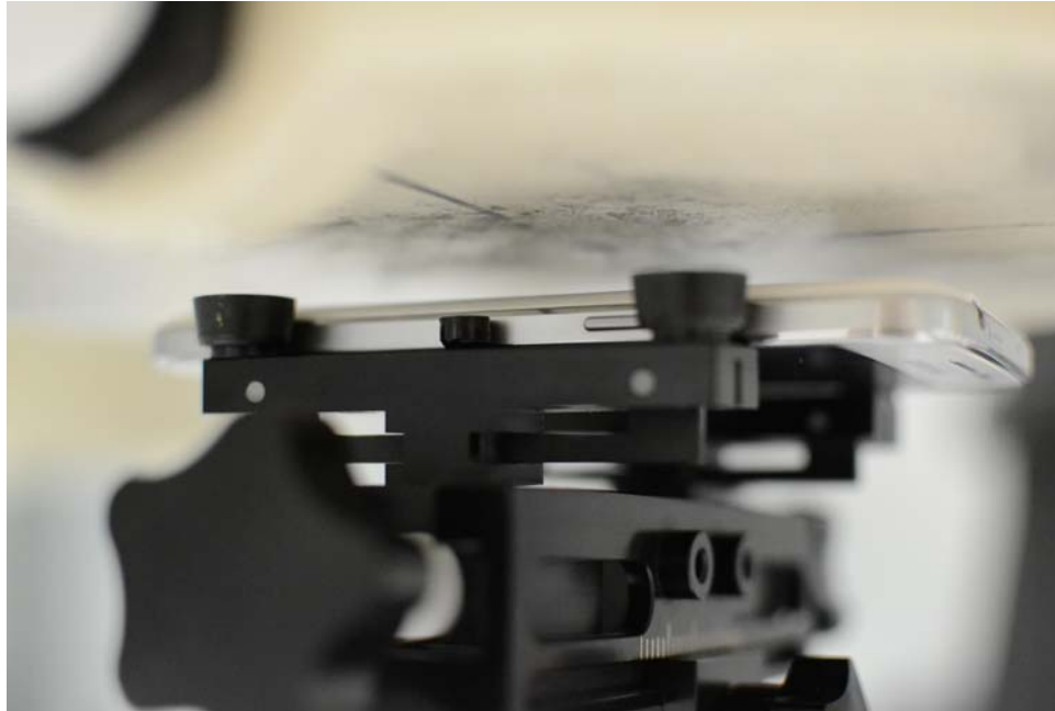
SAR Test Setup Photo 6: Back at 1.0 cm
