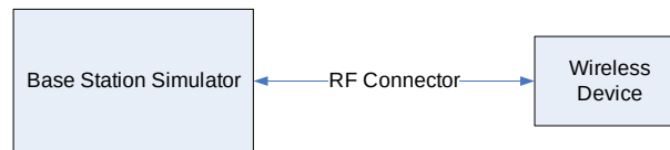
Figure 8-2 Power Measurement Setup
