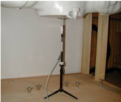
Figure 9-2 System Verification Setup Photo
