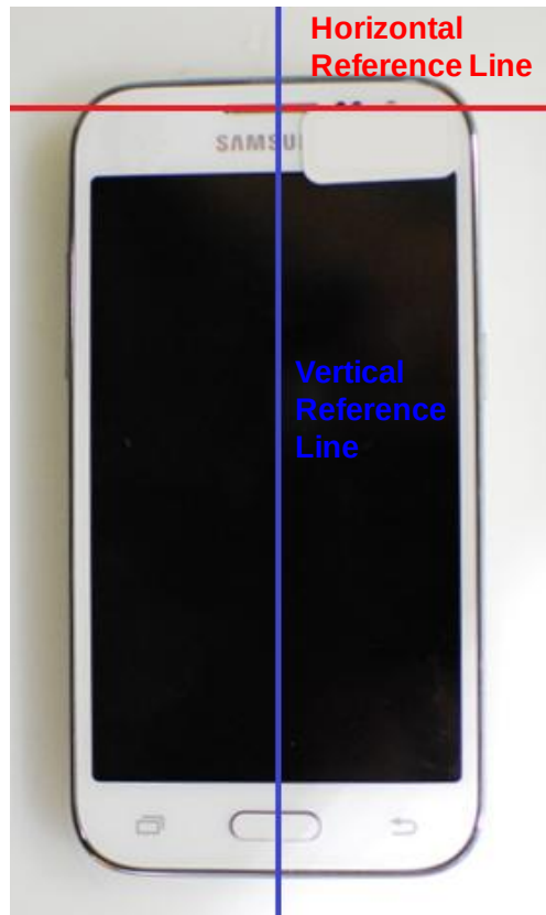
SAR Test Setup Photo 10: Horizontal and Vertical Reference Lines
