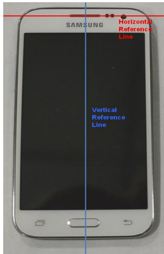
SAR Test Setup Photo 10: DUT Reference Lines
