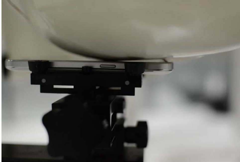
SAR Test Setup Photo 3: Left Cheek
