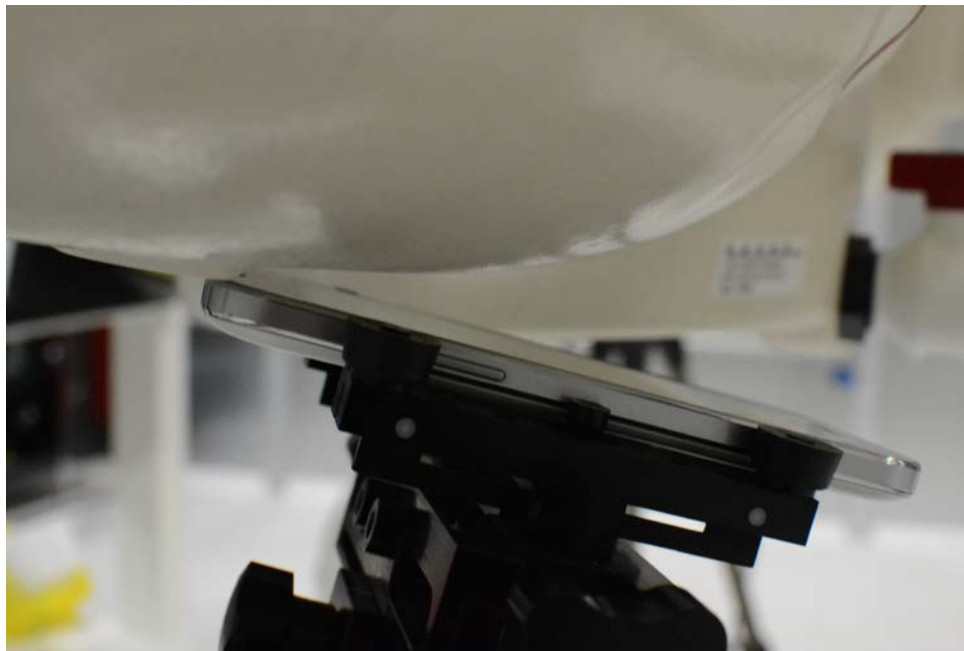
SAR Test Setup Photo 2: Right Tilt
