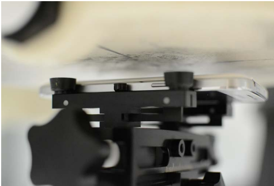
SAR Test Setup Photo 6: Back at 1.0 cm
