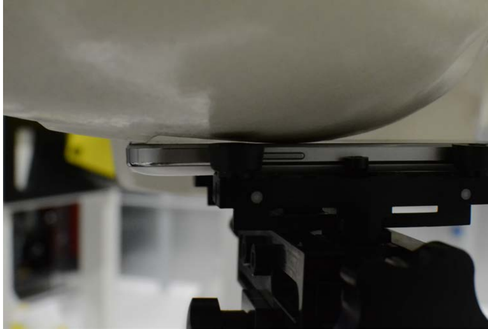
SAR Test Setup Photo 1: Right Cheek
