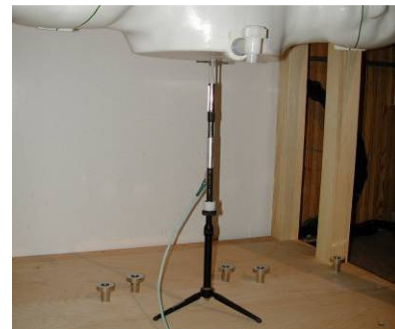
Figure 9-2 System Verification Setup Photo
