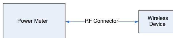
Figure 8-3 Power Measurement Setup
