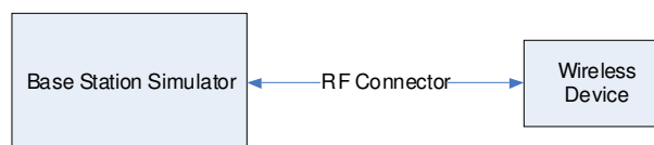
Figure 8-2 Power Measurement Setup
