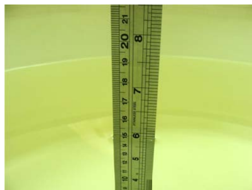
Fig 6.2 Photo of Liquid Height for Body SAR
