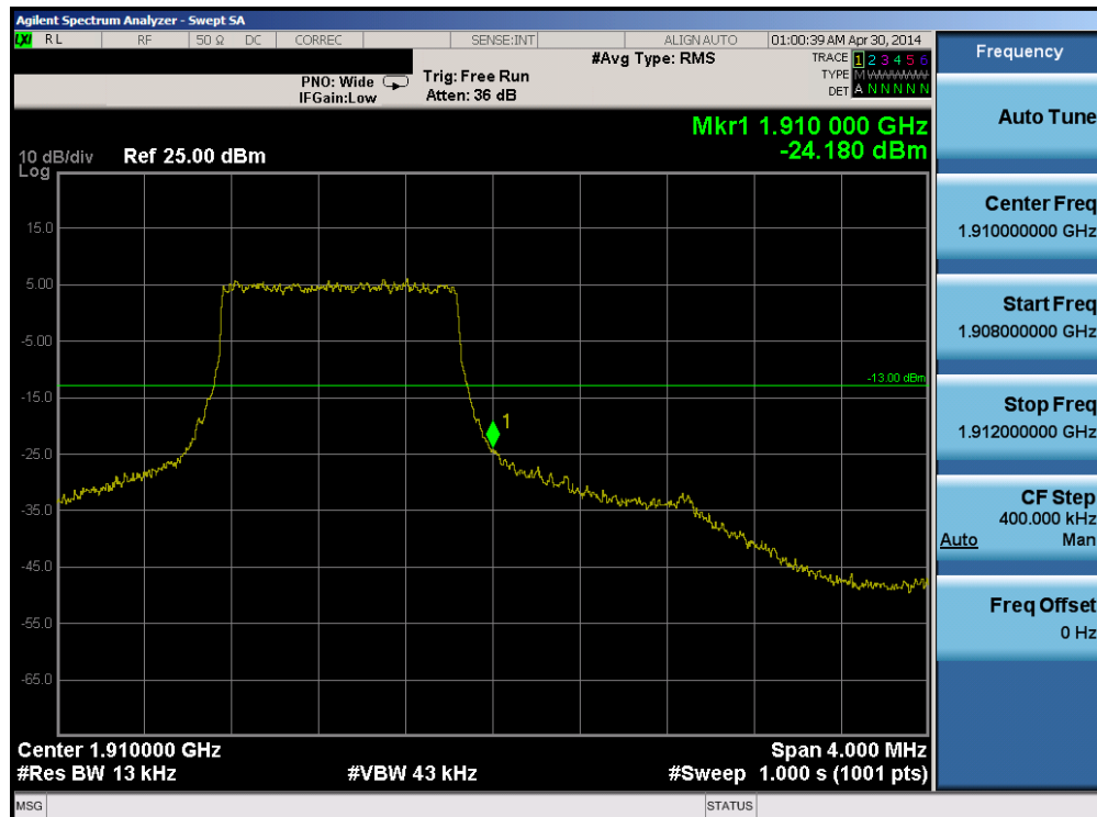
Plot 6-123. Upper Band Edge Plot (Band 2 – 1.4MHz QPSK – RB Size 6)
