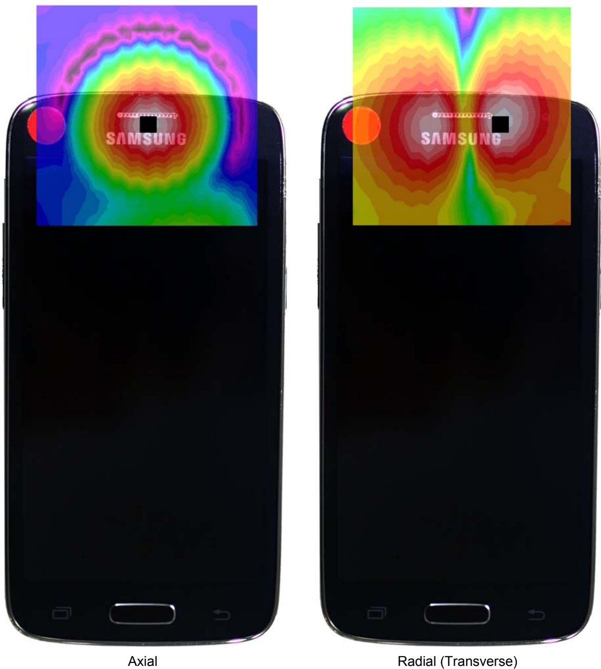
Figure 13-3 T-Coil Scan Overlay Magnetic Field Distributions
