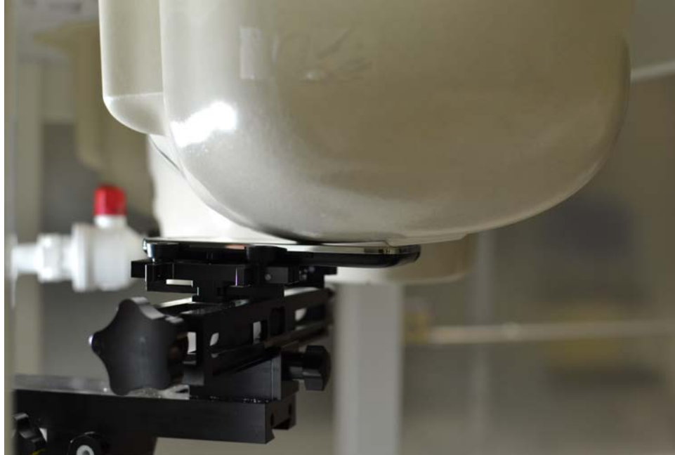
SAR Test Setup Photo 3 – Left Cheek
