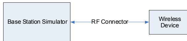
Figure 9-2 Power Measurement Setup
