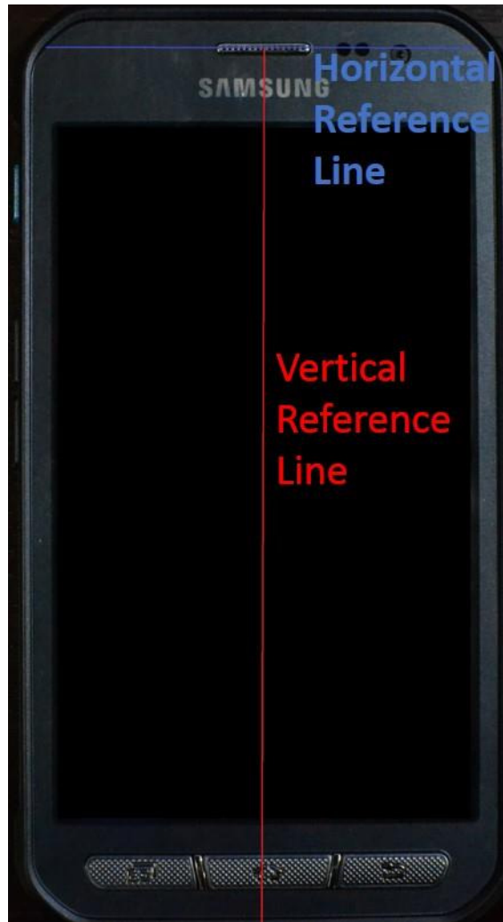
SAR Test Setup Photo 11 – DUT Reference Lines
