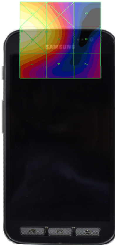
Figure 17-4 E-Field WD Scan overlay
