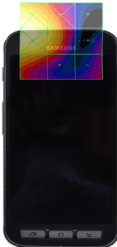
Figure 17-4 E-Field WD Scan overlay
