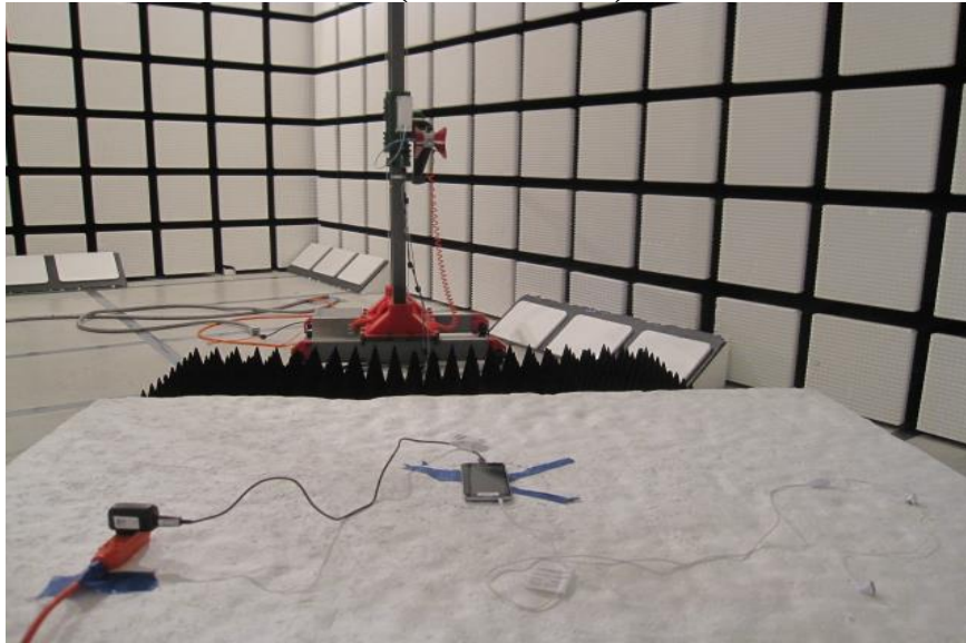
RADIATED BACK PHOTO (ABOVE 1 GHz)
