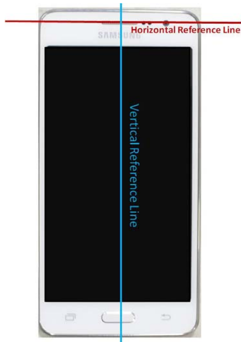
SAR Test Setup Photo 12: DUT reference lines
