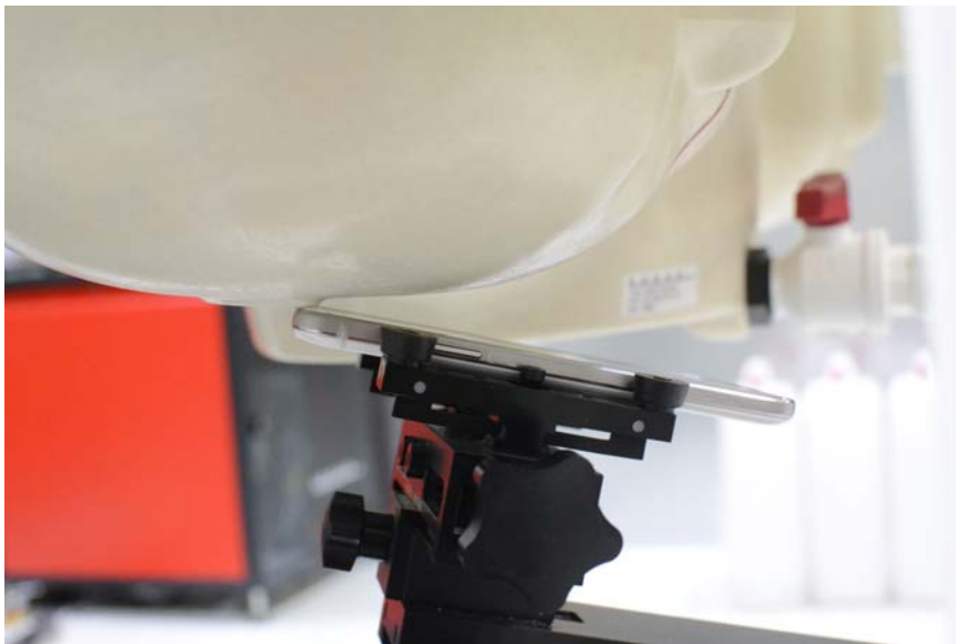
SAR Test Setup Photo 2: Right Tilt
