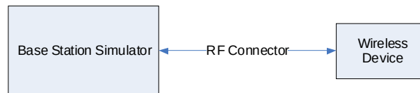
Figure 9-1 Power Measurement Setup
