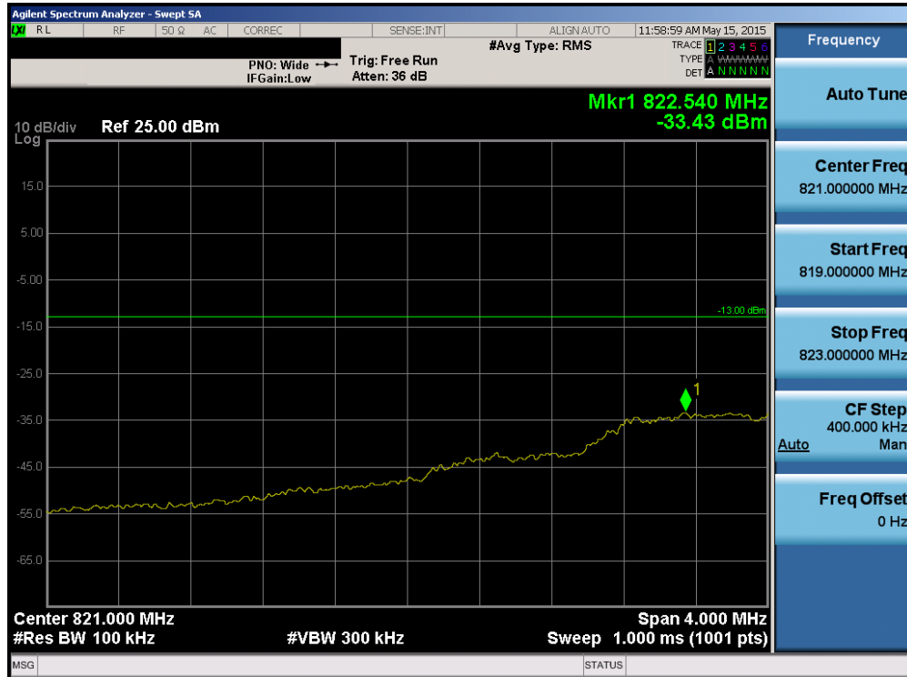
Plot 6-111. Lower Extended Band Edge Plot (Band 5/26 – 1.4MHz QPSK – RB Size 6)
