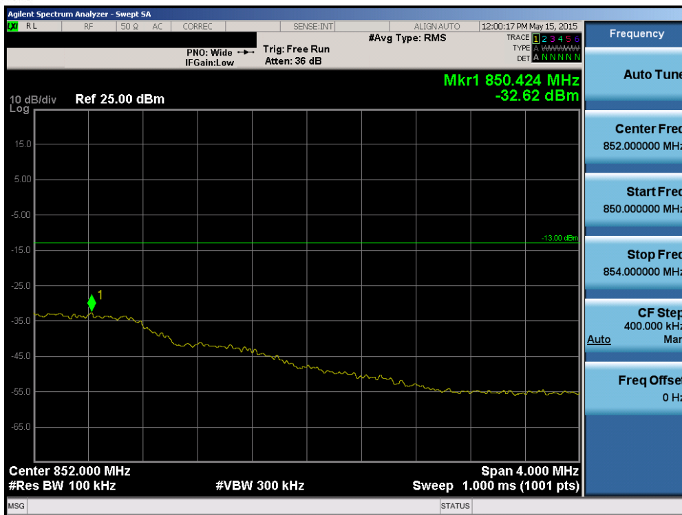
Plot 6-113. Upper Extended Band Edge Plot (Band 5/26 - 1.4MHz QPSK - RB Size 6)
