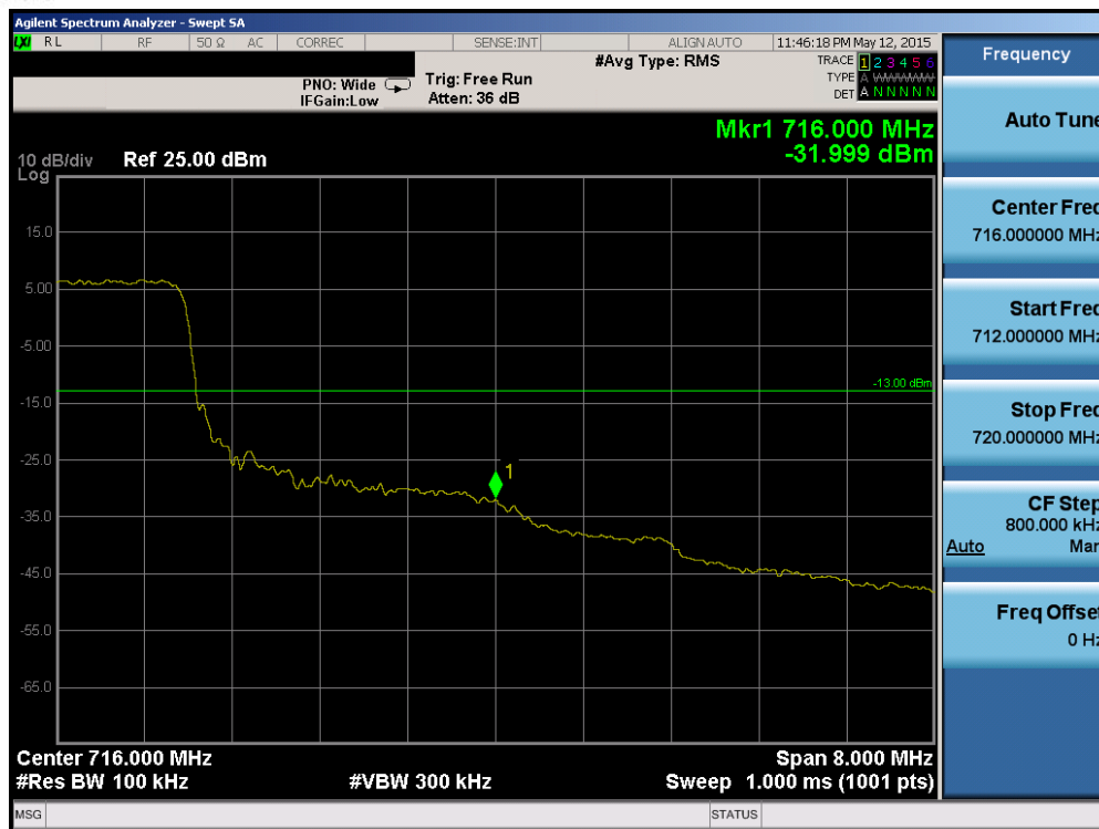
Plot 6-109. Upper Band Edge Plot (Band 12 – 10.0MHz QPSK – RB Size 50)
