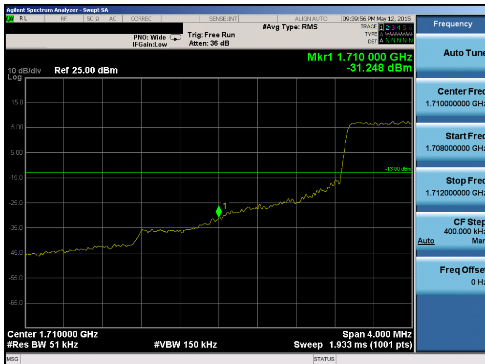
Plot 6-134. Lower Band Edge Plot (Band 4 – 5.0MHz QPSK – RB Size 25)
