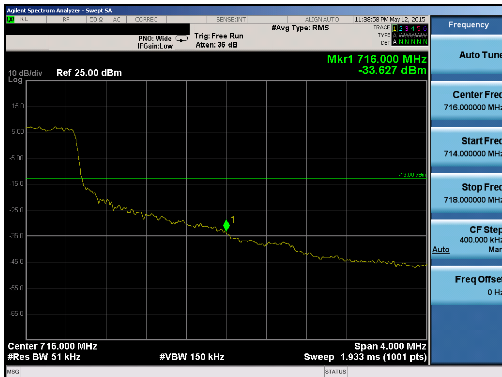
Plot 6-106. Upper Band Edge Plot (Band 12 - 5.0MHz QPSK - RB Size 25)
