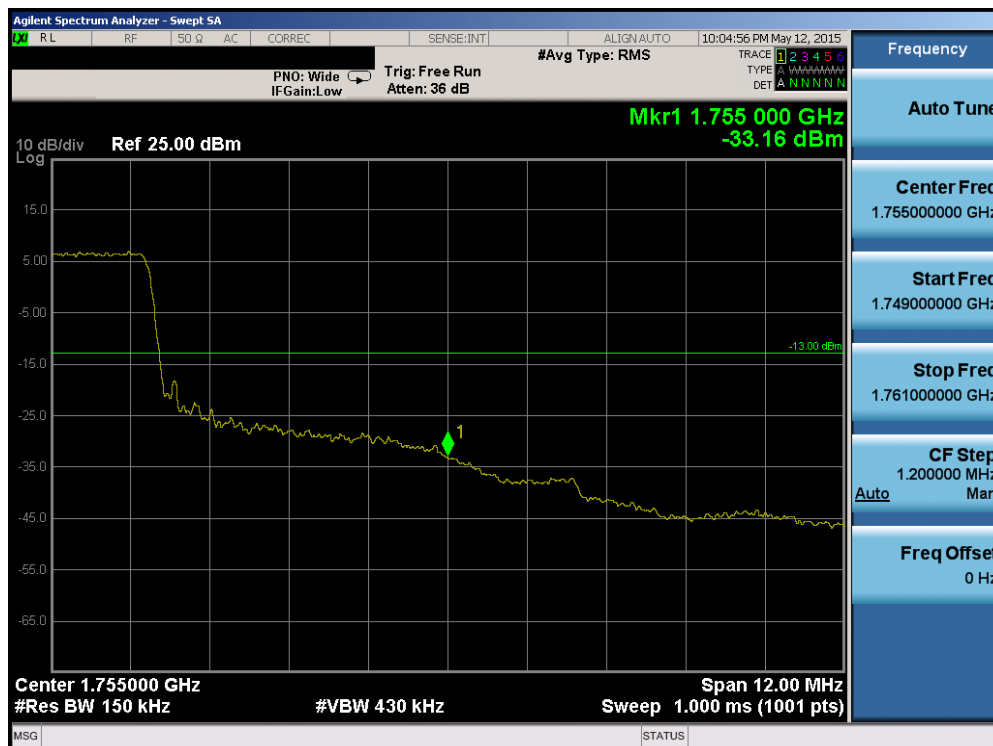
Plot 6-144. Upper Band Edge Plot (Band 4 – 15.0MHz QPSK – RB Size 75)
