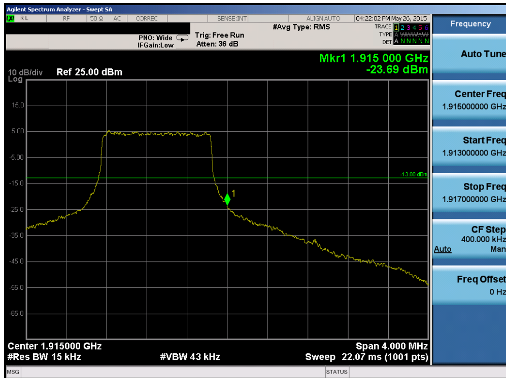
Plot 6-152. Upper Band Edge Plot (Band 2/25 – 1.4MHz QPSK – RB Size 6)
