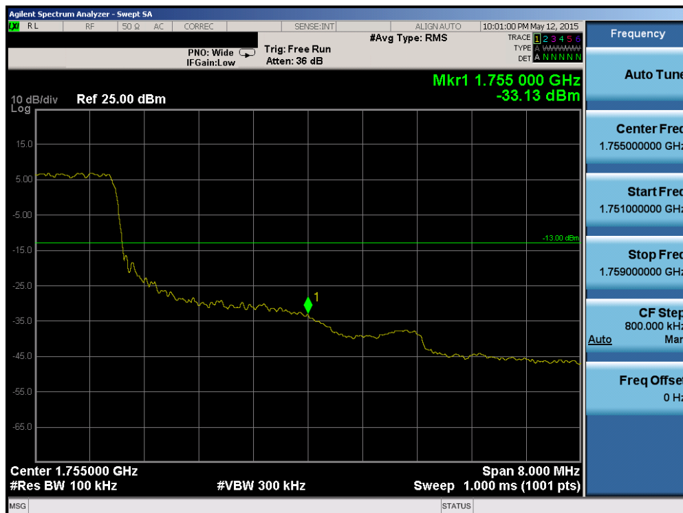
Plot 6-140. Upper Band Edge Plot (Band 4 – 10.0MHz QPSK – RB Size 50)
