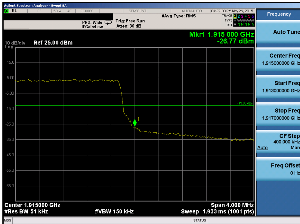
Plot 6-160. Upper Band Edge Plot (Band 2/25 – 5.0MHz QPSK – RB Size 25)
