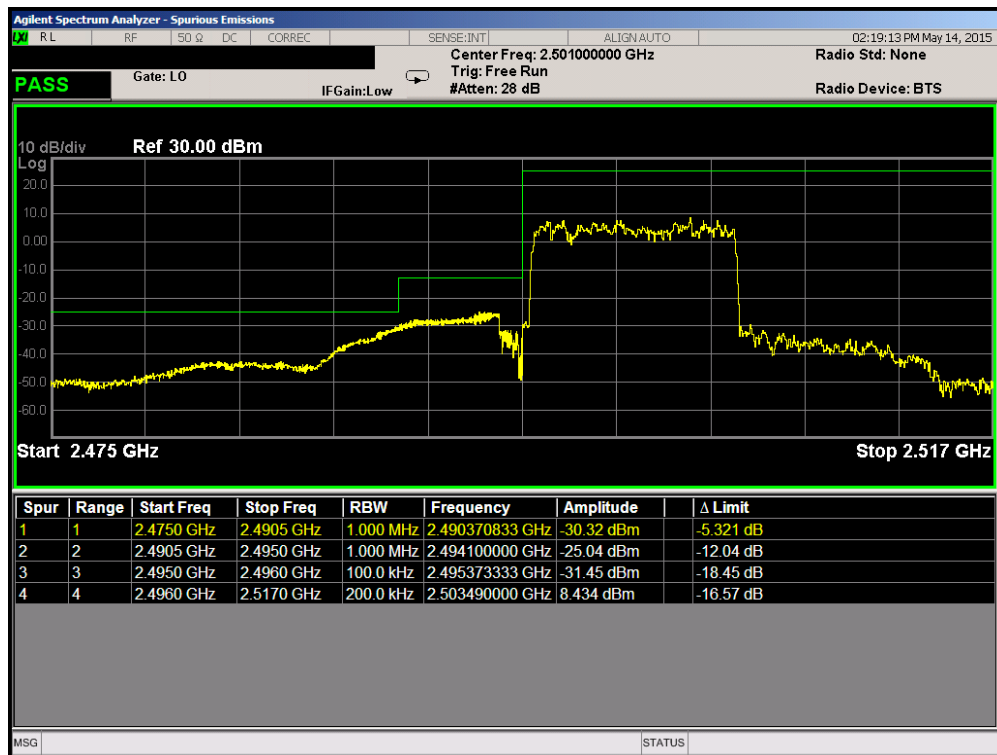
Plot 6-176. Lower ACP Plot (Band 41 – 10.0MHz QPSK – RB Size 50)
