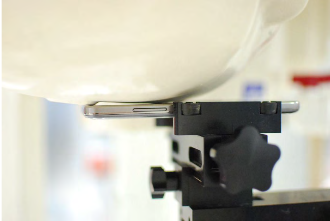
SAR Test Setup Photo 1: Right Cheek
