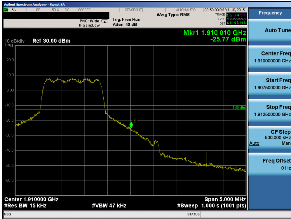
Plot 6-25. Band Edge Plot (PCS CDMA Mode – Ch. 1175)
