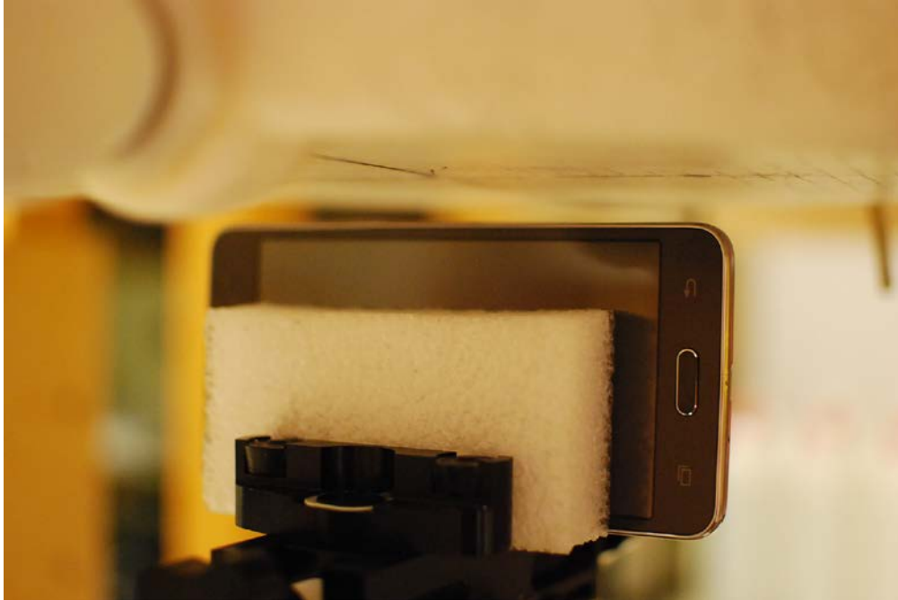
SAR Test Setup Photo 9: Right at 1.0 cm
