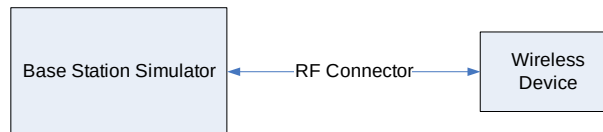
Figure 9-2 Power Measurement Setup
