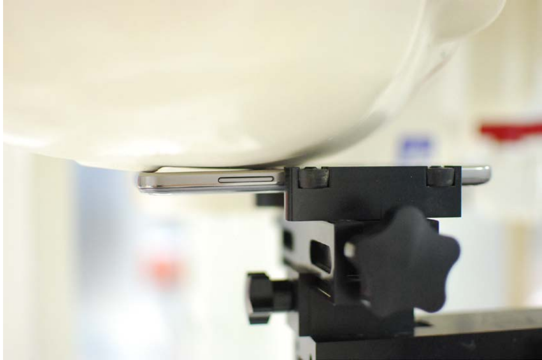
SAR Test Setup Photo 1: Right Cheek
