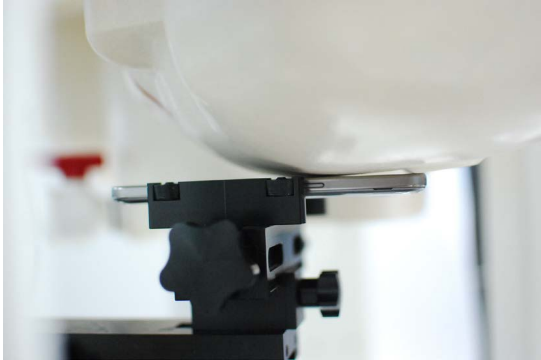
SAR Test Setup Photo 3: Left Cheek
