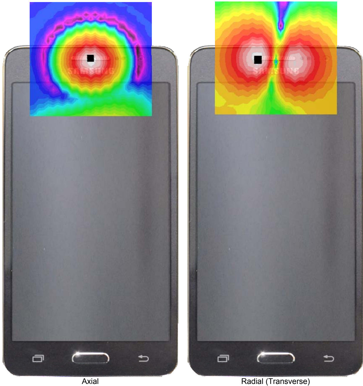
Figure 13-3 T-Coil Scan Overlay Magnetic Field Distributions
